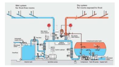
Systems would be a combination of air and water, with the delivery pipework between designated valve sets to the sprinkler head running dry with a compressed air feed. From the monitored valve sets to the sprinkler pumps and tank feeds would be wet.
